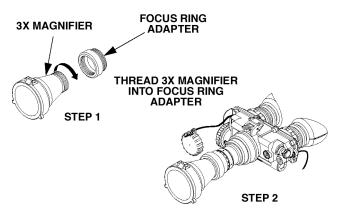
Figure 2-27. 3X Magnifier Installation with LIF in Place.
